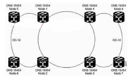
As shown in the exhibit, a customer has several interconnected core rings. They want to create several virtual rings utilizing their STM-64 backbone (Nodes 1, 2, 3, and 4).
