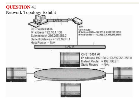
In the DCN connection shown in the exhibit, all non-GNE nodes are located on different subnets from the GNE. There are no static routes or external OSPF on any elements. CTC Workstation and GNE have Router has its default gateway. Can the CTC workstation see the entire SDH network?
