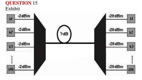
What is the maximum allowable loss budget between the ONS 15216 Mux (left side) composite output and the ONS Demux (right side) composite input, with the optical values given in the exhibit?
