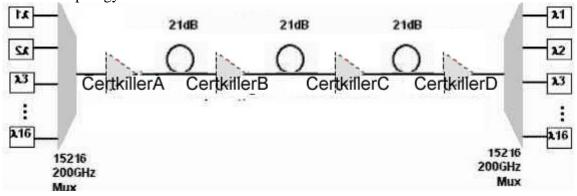
Give the following paramers: Transmitter output (min): -2 dBm Receiver input (min): -28 dBm 15216 Mux and Demux loss: 4.5 dB 16 channels maximum In which sites shown in the exhibit could the 15216 EDFAs be placed to minimize the number of EDFAs needed`?
